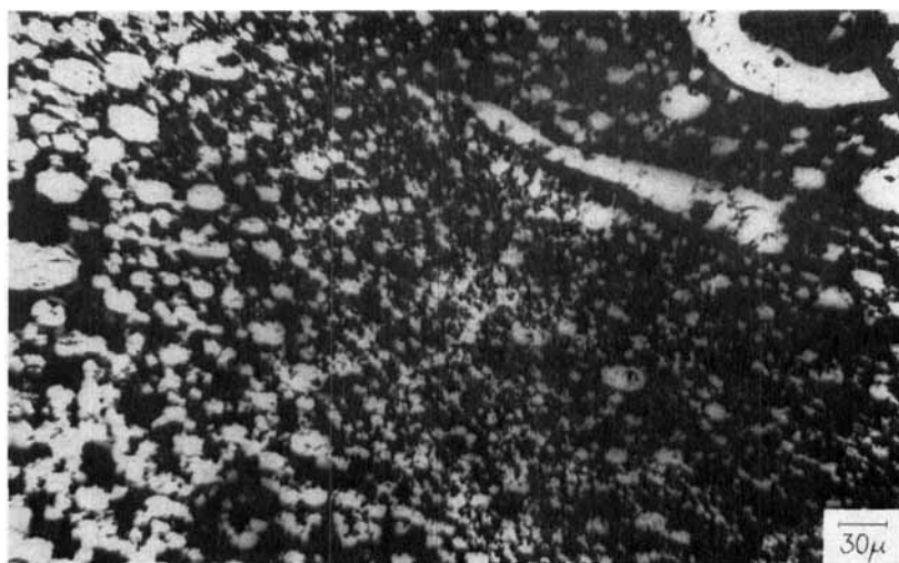
FIGURE 5 Photomicrograph of a cross section of the extrudate obtained from a capillary of 3.23 mm diameter: a—surface layer of extrudate; b—centre of extrudate.
