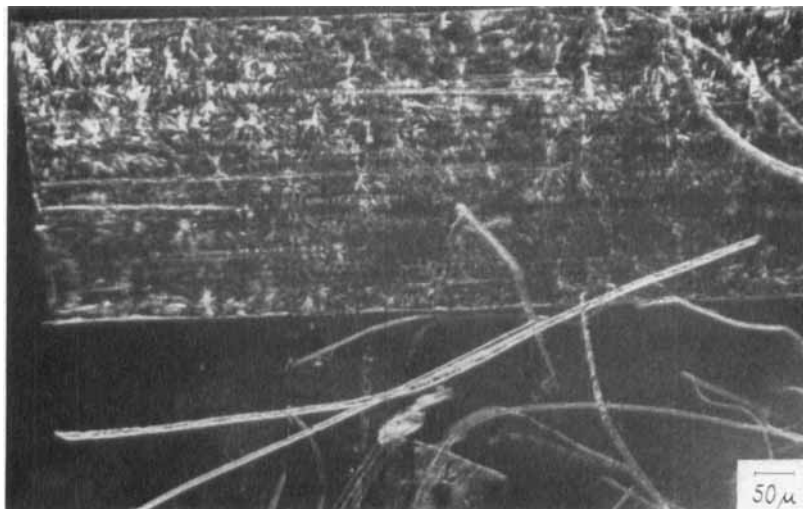
FIGURE 9 The appearance of a polyoxymethylene film contained in a bundle of fibres obtained after the washout of CPA from extrudate. The extrudate is the one obtained after the first extrusion.
