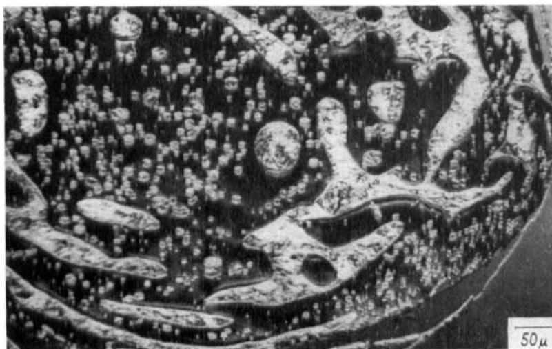
FIGURE 10 Photomicrograph of a lateral section of the extrudate obtained when the time of melting and tempering of a mixture prior to extrusion was 36 min.
