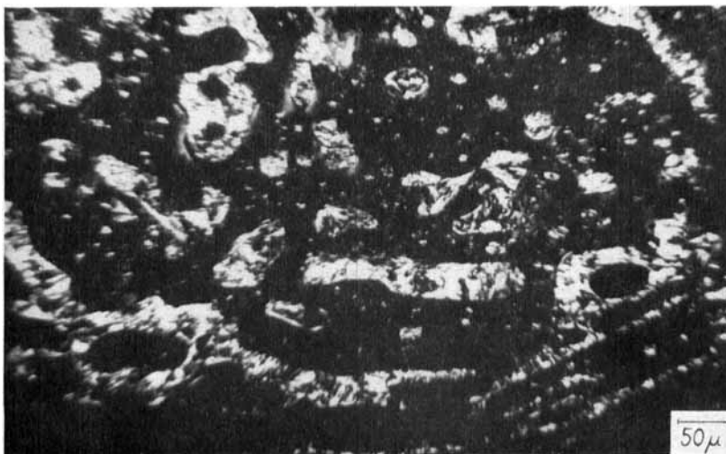
FIGURE 4 Photomicrograph of a cross section of an extrudate of a mixture of POM and CPA. The mixing was carried out from a 10 per cent solution of CPA in ethanol.
