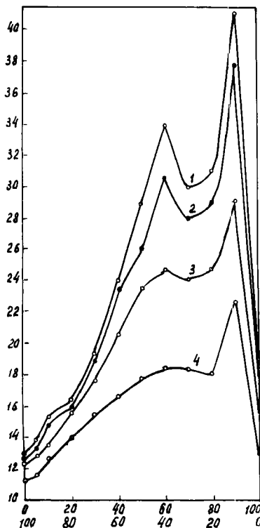
FIGURE 2 The composition dependence of the viscosity of a molten mixture of POM and CPA after the first extrusion through a capillary at t = 190^{\circ}\text{C} . The curves 1–4 correspond, respectively, to the following shear stresses: 0.6, 0.9, 1.8, and 3.5 dynes/cm 2 .
